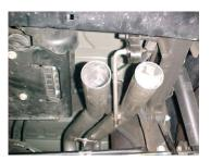
Install the passenger side over axle tailpipe # D into the muffler 1-1/2" to 2". Insert welded hanger into rubber grommet. Use clamp # J to secure pipe to muffler, do not tighten.
