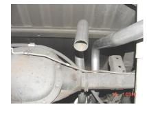
INSTALL DRIVERS SIDE FRONT TAILPIPE # D INTO MUFFLER 1-1/2" TO 2". USE CLAMP # I AND ATTACH IT TO THE MUFFLER. INSERT WELDED HANGER INTO RUBBER GROMMET. DO NOT TIGHTEN.
