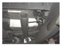
INSTALL HEADPIPE # A USING BOLT KIT # N & #K GASKET. INSERT WELDED HANGER INTO RUBBER GROMMET AND ATTACH TO STOCK FLANGE. DO NOT TIGHTEN.
