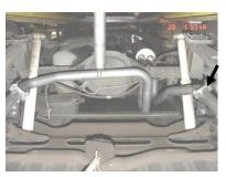
INSTALL DRIVERS SIDE OVERAXLE PIPE # E ONTO FRONT TAILPIPE USING CLAMP #I. USE CLAMP # I TO HOLD TAILPIPE UP TO REAR HANGER # G. DO NOT TIGHTEN. USE ZIP TIES FOR BRAKE LINES.
