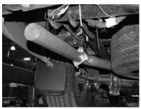
INSTALL DRIVER SIDE TAILPIPE #D INTO MUFFLER AT LEAST 1 ½" TO 2". THIS PIPE WILL ROUTE OVER THE AXLE AND BETWEEN THE SHOCK AND TIRE. ATTACH CLAMP # H TO SECURE PIPE TO MUFFLER. DO NOT TIGHTEN. LOOKING FROM THE REAR OF THE VEHICLE - THIS TAILPIPE IS AT APPX. 11 O'CLOCK.
