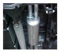
INSTALL MUFFLER #C ONTO HEADPIPES 1  $\frac{1}{2}$ " TO 2". USE CLAMP #G TO SECURE MUFFLER TO HEADPIPES. DO NOT TIGHTEN. OUTLETS SHOULD BE AT THE TOP. SUPPORT MUFFLER WITH A JACK STAND.
