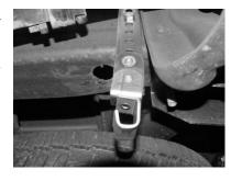
INSTALL METAL HANGERS # J INTO HOLES LOCATED APPROX. 16" FROM THE REAR OF THE FRAME. METAL HANGERS ARE MOUNTED ON THE OUTSIDE OF FRAME. USE THE HARDWARE THE PROVIDED. THE BOLT AND WASHER WILL GO INTO THE 1ST HOLE FROM THE TOP OF THE HANGER.
