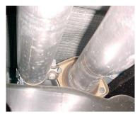
REMOVE YOUR STOCK EXHAUST FROM THE FACTORY FLANGES LOCATED JUST BEHIND YOUR FACTORY Y-PIPE. NEXT CUT OFF YOUR TAILPIPE JUST BEHIND THE MUFFLER. USE WD-40 TO AID IN THE REMOVAL OF RUBBER GROMMETS FROM HANGERS.
