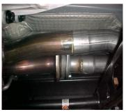
INSTALL PASSENGERSIDE HEADPIPE #A ONTO FACTORY FLANGE USING THE HARDWARE KIT # K. DO NOT TIGHTEN. INSERT HANGER INTO RUBBER GROMMET. NEXT, INSTALL DRIVERSIDE HEADPIPE #B ONTO THE FACTORY PIPE. USE CLAMP # I TO SECURE. DO NOT TIGHTEN.
