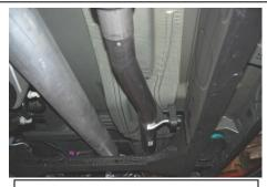
3. Install muffler assembly Item # B onto the head pipe 6". You may need to use a jack stand to support the muffler while installing the tailpipe. Use Item# E to clamp the muffler assembly to the head pipe. Loosely tighten down.
