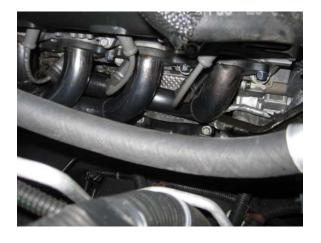
10) WRAP SPARK PLUG BOOT WITH HEAT WRAP PROVIDED AND RE-INSTALL. USING THE NUTS AND BOLTS PROVIDED, RECONNECT THE HEADERS TO THE STOCK EXHAUST UNDERNEATH THE VEHICLE.
