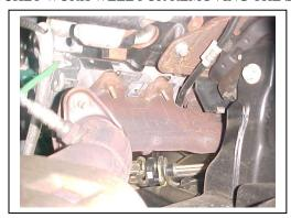
6. THE DIPSTICK MUST NOW BE REMOVED. IT HAS A SEPARATE MOUNTING BOLT ON THE HEAD AND USES AN O-RING SEAL AT THE BOTTOM. USE CARE TO PROTECT THE O-RING.
