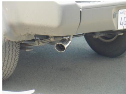
INSTALL THE STAINLESS STEEL TIP. TO CLEAN TIP USE ANY STAINLESS OR ALUMINUM CLEANER AND A SCOTCH BRITE PAD. NOW GO BACK AND TIGHTEN ALL CLAMPS, NUTS AND BOLTS STARTING FROM THE FRONT AND WORKING YOUR WAY BACK.
