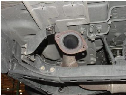
INSTALL HEADPIPE #A ONTO STOCK FLANGE, RE-USING YOUR STOCK GASKET, NUTS AND BOLTS. DO NOT TIGHTEN. JUST SNUG IT UP. INSERT HANGER INTO RUBBER GROMMET.
