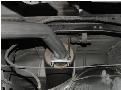
INSTALL MUFFLER #B ONTO HEADPIPE #A WITH INLET TOWARDS THE MOTOR. USE CLAMP #F TO SECURE MUFFLER TO THE HEADPIPE. DO NOT TIGHTEN. OUTLET OF MUFFLER SHOULD BE AT THE 5 O'CLOCK POSITION. INSTALL HANGER #E AND INSERT HANGER INTO RUBBER GROMMET. DO NOT TIGHTEN. INLET OF MUFFLER IS LOOKING INTO THE LOUVERS.
