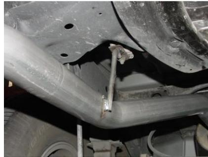
INSTALL TAILPIPE #C ONTO MUFFLER 1-1/2" TO 2". ROTATE TAILPIPE UNTIL REAR HANGER LINES UP WITH THE FACTORY GROMMET. INSTALL HANGER WITH FACTORY NUT THAT YOU REMOVED FROM STOCK EXHAUST. ROTATE TAILPIPE UNTIL YOU HAVE CLEARANCE FROM THE SHACKLE AND LEAF SPRING.
