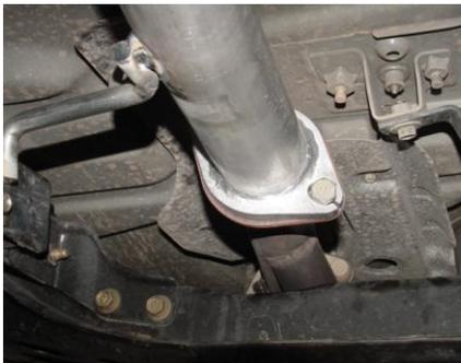
INSTALL THE HEADPIPE RE-USING THE FACTORY GASKET AND BOLTS. APPLY A SMALL AMOUNT OF HI-TEMP GASKET SEALER ONTO THE GASKET TO ENSURE A LEAK FREE CONNECTION. DO NOT TIGHTEN. INSTALL HEADPIPE HANGER USING ONE OF THE FACTORY NUTS AND BOLT #F.
