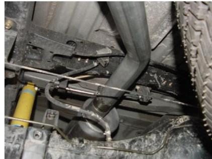
SLIP THE OVER AXLE TAILPIPE #C INTO THE OUTLET OF THE MUFFLER 1" TO 2". CONNECT REAR HANGER WITH FACTORY BOLT. INSERT WELDED HANGER INTO RUBBER GROMMET. USE CLAMP #D TO SECURE TAILPIPE TO THE MUFFLER. DO NOT TIGHTEN.
