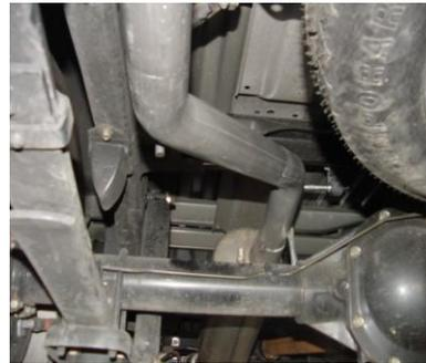
INSTALL TAILPIPE #C INTO MUFFLER 1-1/2" TO 2". INSERT WELDED HANGER INTO RUBBER GROMMET. USE CLAMP #E TO SECURE TAILPIPE TO MUFFLER. DO NOT TIGHTEN. INSTALL THE REAR HANGER USING THE FACTORY NUT.
