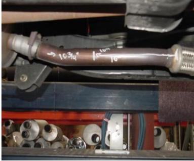
LAY OUT THE GIBSON EXHAUST ON THE FLOOR AND COMPARE PART NUMBERS WITH THE DRAWING. **TO REMOVE STOCK EXHAUST MEASURE 10 3/4" FROM THE FRONT OF THE MUFFLER TOWARDS THE MOTOR**, CUT THE TAILPIPE OFF IN THAT SPOT. REMOVE THE REAR HANGER AND SAVE THE FACTORY HARDWARE YOU WILL RE-USE IT. LEAVE ALL RUBBER GROMMETS ON THE HANGER. USE WD-40 TO AID IN REMOVAL OF THE EXHAUST AND HANGERS.
