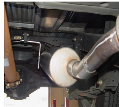
INSTALL MUFFLER #B ONTO HEADPIPE 1-1/2" TO 2". OUTLET OF MUFFLER SHOULD BE AT THE 3 O'CLOCK POSITION. USE CLAMP #E TO SECURE MUFFLER TO THE HEADPIPE. DO NOT TIGHTEN. MUFFLER INLET IS LOOKING INTO THE LOUVERS.
