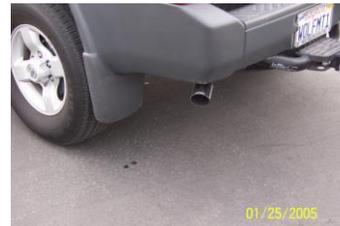
**MAKE SURE YOU HAVE A 1" CLEARANCE ON ALL PIPES FROM BRAKE & FUEL LINES, TIRES, SHOCKS, ETC...**
