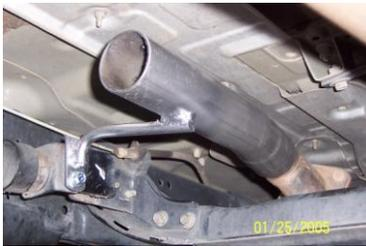
INSTALL HEADPIPE #A ONTO STOCK PIPE, USE CLAMP # E TO SECURE PIPES TOGETHER. DO NOT TIGHTEN. NEXT, MOUNT WELDED HANGER TO RUBBER GROMMET USING BOLT KIT # F.
