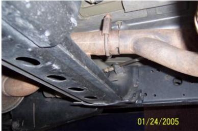
TO REMOVE STOCK EXHAUST, REMOVE IT FROM THE CLAMP LOCATED IN FRONT OF YOUR STOCK MUFFLER. NEXT REMOVE THE FACTORY 12 MM NUT ON THE REAR TAILPIPE. DO NOT DISCARD YOU WILL REUSE IT.
