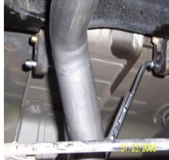
INSTALL TAILPIPE #C ONTO MUFFLER 1-1/2" TO 2". ROTATE TAILPIPE UNTIL REAR HANGER LINES UP WITH THE FACTORY GROMMET. INSTALL WELDED HANGER WITH FACTORY 12MM NUT THAT YOU REMOVED FROM STEP #1. INSERT OTHER WELDED HANGERS INTO RUBBER GROMMETS. USE CLAMP #E TO SECURE TAILPIPE TO MUFFLER. DO NOT TIGHTEN.
