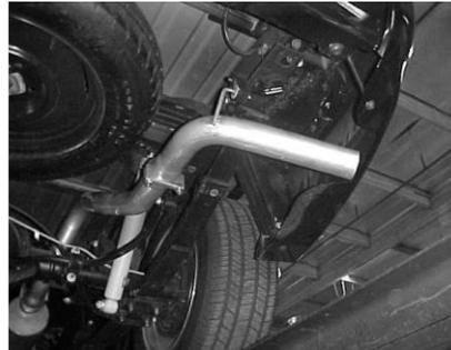
4. BEFORE INSTALLING OVERAXLE TAILPIPE, THE FACTORY REAR TAILPIPE HANGER MUST BE UNBOLTED AND ROTATED 180 DEGREES. Insert the overaxle tailpipe. #C no less than  $1\frac{1}{2}$ " and no more than 2". Slightly lean to the driver side. Slide turnout pipe #D on to the tailpipe. Roll turnout pipe until you have it at the correct angle for your truck. Insert welded hanger into rubber grommet. Clamp down. Using clamp #H
