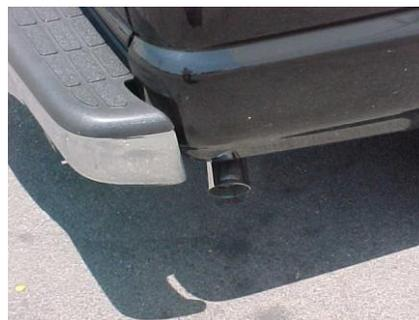
5. Install stainless steel tip. Clamp down. To clean stainless steel tip use any stainless or aluminum cleaner. When you have everything in place, tighten all bolts and clamp down.
