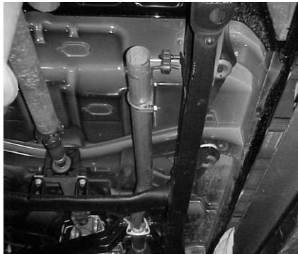
2. Bolt on front headpipe #A re-using factory bolts and gasket #I. Use a RTV gasket sealer for flange connection. (Note Headpipe will lean toward passenger side.) Install hanger #F onto the front headpipe and insert into rubber grommet.
