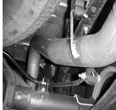
INSTALL THE OVER AXLE PIPE #C INTO MUFFLER NO LESS THEN 1-1/2" AND NO MORE THAN 2" .SLIP REAR WELDED HANGER INTO THE FACTORY RUBBER GROMMET. ATTACH TO MUFFLER WITH CLAMP #H.
