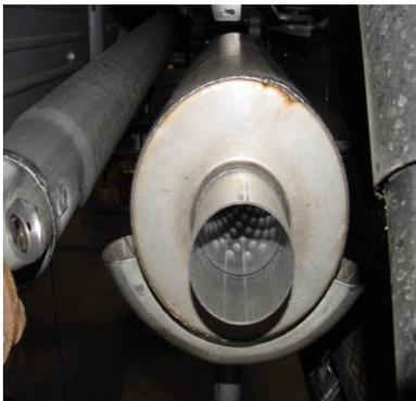
SLIDE MUFFLER WITH BAFFLES FACING FORWARD TOWARDS CONVERTER ONTO THE HEADPIPE NO LESS THEN 1 1/2" AND NO MORE THAN 2". MUFFLER INLET IS LOOKING INTO LOUVERS.
