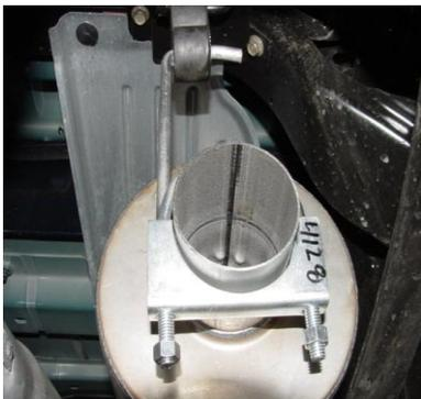
USE HANGER #F AT THE REAR OF THE MUFFLER WITH VERTICAL BAR OF HANGER ON PASSENGER SIDE AND INSERT WELDED ROD INTO RUBBER GROMMET. DO NOT TIGHTEN.
