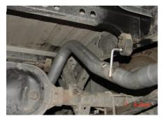
INSTALL TAILPIPE #C INTO MUFFLER 1-1/2" TO 2". INSERT WELDED HANGER INTO RUBBER GROMMET.
