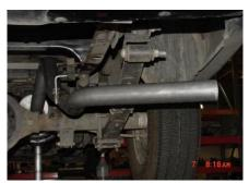
INSTALL EXITPIPE #D ONTO TAILPIPE. ROTATE THE PIPE UNTIL IT IS LEVEL. USE CLAMP #H TO SECURE. DO NOT TIGHTEN.
