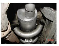
INSTALL MUFFLER #B ONTO HEADPIPE 1-1/2" TO 2" WITH THE INLET FACING THE MOTOR. ROTATE MUFFLER UNTIL THE OUTLET IS AT THE 6 O'CLOCK POSITION. THE INLET OF THE MUFFLER IS LOOKING INTO THE LOUVERS.
