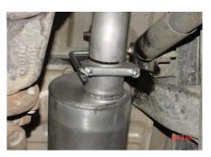
INSTALL REAR MUFFLER HANGER #F INTO RUBBER GROMMET JUST ABOVE THE OUTLET OF THE MUFFLER. THE END OF THE HANGER WILL POINT TOWARDS THE PASSENGER SIDE OF THE VEHICLE. DO NOT TIGHTEN.
