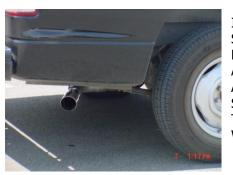
INSTALL THE STAINLESS TIP. NOW GO BACK AND TIGHTEN ALL CLAMPS STARTING IN THE FRONT AND WORKING BACK.
