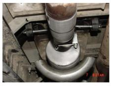
INSTALL FRONT MUFFLER HANGER #G INTO THE RUBBER GROMMETS LOCATED JUST ABOVE THE INLET OF THE MUFFLER. THIS CLAMP WILL BE USED TO SECURE THE MUFFLER TO THE HEADPIPE. DO NOT TIGHTEN.
