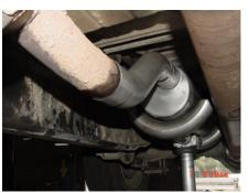
TO REMOVE STOCK EXHAUST UNBOLT THE CLAMP LOCATED JUST BEHIND THE CONVERTER. YOU MAY NEED TO HEAT IT UP FOR EASIER REMOVAL. CUT STOCK TAILPIPE OFF BEHIND THE MUFFLER & REMOVE. LEAVE ALL RUBBER GROMMETS ON THE HANGER. USE WD-40 TO AID IN THE REMOVAL OF EXHAUST AND
