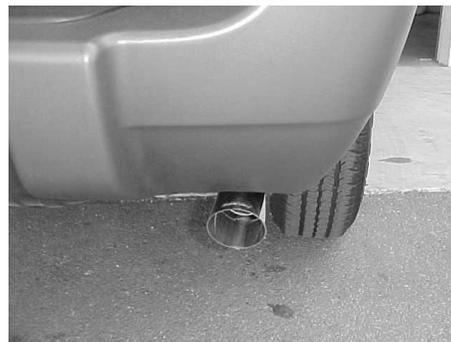
INSTALL YOUR STAINLESS TIP TO YOUR DESIRED LOOK. TO CLEAN TIP USE ANY ALUMINUM OR STAINLESS CLEANER AND A SCOTCH BRITE PAD. NOW TIGHTEN ALL CLAMPS STARTING FROM THE FRONT AND WORKING BACK.
