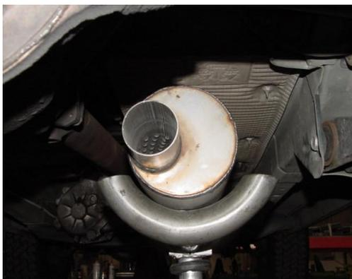
INSTALL REAR MUFFLER HANGER #E VERTICAL ROD ON HANGER #E WILL BE ON DRIVERS SIDE. INSTALL MUFFLER #A ONTO STOCK FRONT PIPE AND ATTACH WITH CLAMP #F. OUTLET SHOULD BE AT THE 9 O'CLOCK POSITION. USE A JACK STAND TO SUPPORT THE MUFFLER. DO NOT TIGHTEN. MUFFLER INLET IS LOOKING INTO THE LOUVERS.
