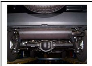
**4.** Install muffler onto head pipe #A 1½"-2" with the louvers facing towards the inlet. Use a jack stand to support the muffler. Use clamp #E to secure the muffler to the headpipe. Do not tighten. Muffler inlet is looking into the louvers.
