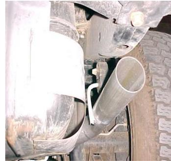
INSTALL TAILPIPE # B INTO MUFFLER 1 1/2" - 2". INSERT WELDED HANGER INTO RUBBER GROMMET, ROTATE PIPE SO YOU HAVE PROPER CLEARANCE. USE CLAMP # D TO SECURE PIPE TO MUFFLER. DO NOT TIGHTEN.
