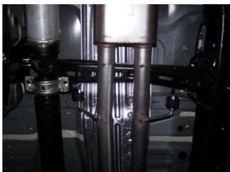
5. Install muffler #C onto headpipes 1.5"-2" with the louvers facing towards the converter. Use a jack stand to support the muffler. Use clamps #G to secure the muffler to the headpipe. Do not tighten. Muffler inlet is looking into the louvers.
