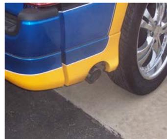
NEXT INSTALL YOUR STAINLESS STEEL TIP TO YOUR DESIRED LOOK. USE ANY ALUMINUM OR STAINLESS STEEL CLEANER TO POLISH YOUR TIP. MAKE SURE YOU HAVE A MINIMUM OF A 1" CLEARANCE ON ALL PIPES FROM ALL RUBBER BRAKE LINES, TIRES, SHOCKS, FUEL LINES, ETC. THEN TIGHTEN ALL CLAMPS AND HANGERS
