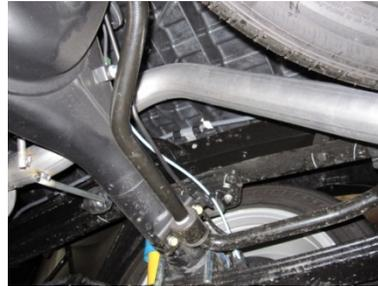
INSTALL THE OVERAXELE TAILPIPE #C INTO THE MUFFLER 1-1/2" TO 2". DO NOT TIGHTEN.
