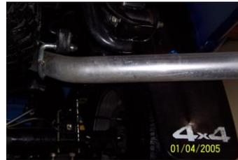
INSTALL MUFFLER #B ONTO HEAD PIPE 1-1/2" TO 2" WITH THE LOUVERS FACING TOWARDS THE CONVERTER. THE MUFFLER OUTLET SHOULD BE POSITIONED AT 12:00. USE A JACK STAND TO SUPPORT THE MUFFLER. USE CLAMP #E TO SECURE THE MUFFLER TO THE HEAD PIPE. DO NOT TIGHTEN. MUFFLER INLET IS LOOKING INTO THE LOUVERS.
