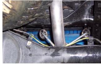
INSTALL THE OVERAXLE TAILPIPE #C INTO THE MUFFLER 1-1/2" TO 2". INSERT WELDED HANGERS INTO RUBBER GROMMET. SECURE TO THE MUFFLER USING CLAMP #E. DO NOT TIGHTEN.
