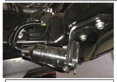
2. Before installing the Gibson exhaust you will need to remove the factory trailer wiring connector and wiring loom bracket seen in the photo above. Please Zip tie the two plug up and away from the exhaust. This will not be re used. Remove your factory spare tire. It will not be re installed.
