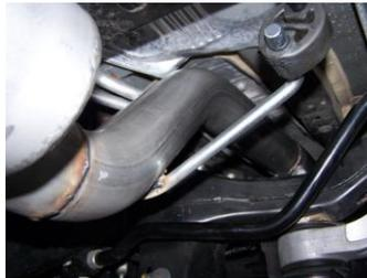
5. Install rear extension pipe #D onto muffler. Insert welded hanger into rubber grommet. Use clamp #H to secure the pipe. Do not tighten.
