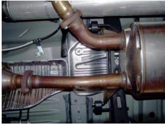
2. Remove the stock exhaust at the 2-bolt flange located in front of the muffler. Dis-engage the welded hangers from the OEM rubber grommets. Use WD-40 to help in the process. Do not damage or remove the rubber grommets as you will reuse them to mount your new system. Now, unbolt the tailpipe and remove exhaust. Do not throw away stock flange bolts, as you will reuse them.
