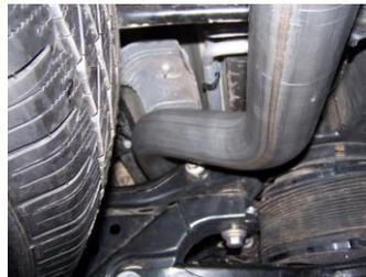
6. Install the over axle tailpipe #E to the rear extension pipe. Use clamp #H to secure pipe. Do not tighten. Install welded hanger into rubber grommet.
