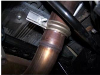
3. Install passenger side headpipe #A using your stock bolts. Do not tighten. Next, install driver side headpipe #B using stock bolts. Do not tighten. Insert welded hangers into rubber grommets.
