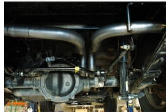
7. Install stainless steel tips. Clamp down. When you have everything in place, firmly tighten all bolts and clamps down securely. Use stainless steel or aluminum cleaner to polish tips. Inspect all fasteners after 25-50 miles of operation and re-tighten as necessary.
