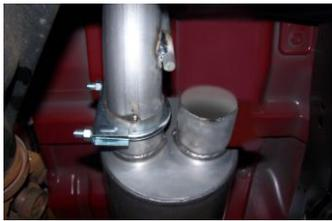
4. Slide driver side over axle tailpipe #B into muffler 1.5-2". Use clamp #F to secure tailpipe to muffler. Do not tighten. Insert welded hanger into rubber grommet.
