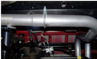
5. Slide the second driver side over axle tailpipe #C onto pipe #B 1.5-2". Secure pipes using clamp #F. Do not tighten. Insert welded hanger into rubber grommet.
