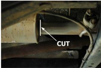
2. To remove the stock exhaust, cut just in front of the stock resonator. (see picture) Disengage the welded hangers from the OEM rubber grommets. Use WD-40 to aid in the process. Do not damage or remove the rubber grommets as they will be reused to mount the new system. Now, cut off tailpipe and remove exhaust.
