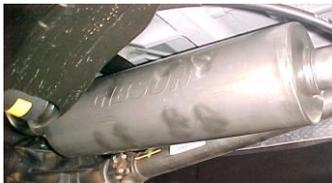
3. Slide muffler #A onto headpipe 1½"-2". Use a jack stand to support the muffler. Make sure muffler outlets are level. Use clamp #G to secure the muffler to the headpipe. Do not tighten.
