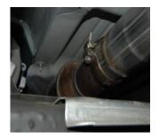
3. Install headpipe #A onto and attach using stock hardware. Do not tighten. Insert welded hanger into
