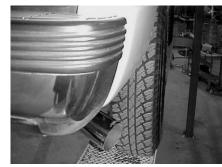
INSTALL TURNOUT PIPE #D INTO TAILPIPE USING CLAMP #F . INSTALL THE STAINLESS TIP AND CLAMP DOWN. USE ANY STAINLESS STEEL OR ALUMINUM CLEANER TO POLISH TIP.
