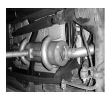
SLIDE MUFFLER #B WITH DUAL INLET ONTO HEADPIPE AT LEAST 1-1/2" TO 2". MUFFLER OUTLET SHOULD BE AT THE 12 O'CLOCK POSITION. USE CLAMPS #F TO ATTACH HEADPIPE. MAKE SURE INLETS AND MUFFLER IS LEVEL. AND TIGHTEN DOWN. USE JACK STAND TO SUPPORT MUFFLER.
