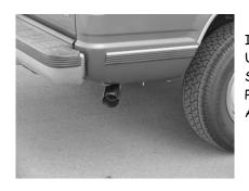
MAKE SURE YOU HAVE A 1" CLEARANCE ON ALL PIPES FROM ALL RUBBER BRAKE LINES, FUEL LINES, SHOCK BOOTS, TIRES, ETC
