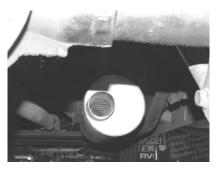
SLIDE MUFFLER # B ONTO HEADPIPE AT LEAST 1"- 2" WITH INLET TOWARDS THE MOTOR. OUTLET SHOULD BE AT 9 O'CLOCK POSITION. INLET OF MUFFLER IS LOOKING INTO THE LOUVERS. USE A JACKSTAND TO SUPPORT THE MUFFLER.
