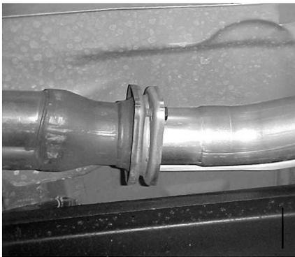
UNBOLT THE STOCK EXHAUST AT THE FLANGE BEHIND THE Y-PIPE AND REMOVE. MAKE SURE TO LEAVE ALL RUBBER GROMMETS IN THE FACTORY LOCATION. **YOU WILL RE-USE STOCK NUTS, BOLTS.** FOR EASIER REMOVAL OF EXHAUST, CUT BEHIND THE MUFFLER. USE WD-40 TO REMOVE HANGERS FROM GROMMETS.
