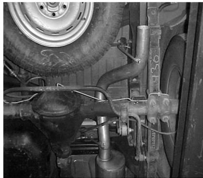
INSTALL OVERAXLE TAILPIPE #C TO THE OUTLET OF THE MUFFLER USING HANGER #G. INSERT WELDED HANGER INTO RUBBER GROMMET.
