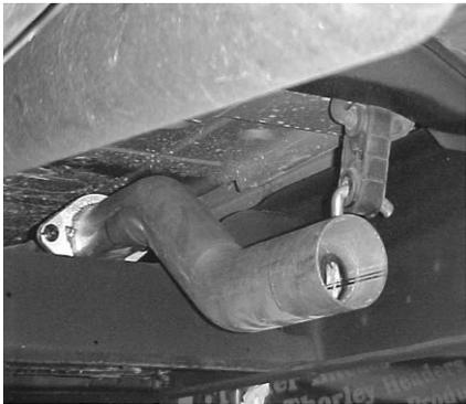
BOLT HEADPIPE #A TO THE STOCK FLANGE RE-USING THE FACTORY NUTS, BOLTS AND GASKET # H. INSERT WELDED HANGER INTO RUBBER GROMMET.
