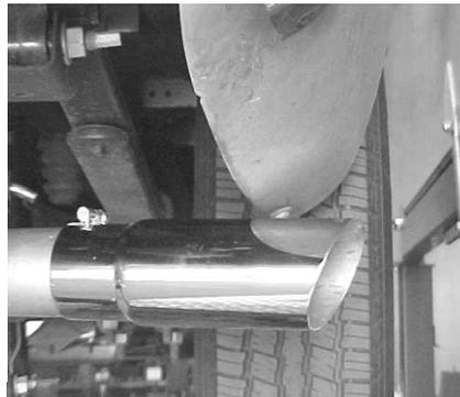
INSTALL THE STAINLESS STEEL TIP NOW; FIRMLY TIGHTEN EVERYTHING ALL CLAMP, HANGERS, BOLTS AND FLANGE. TO CLEAN TIP USE ANY STAINLESS OR ALUMINUM CLEANER WITH A SCOTT BRITE PAD.
