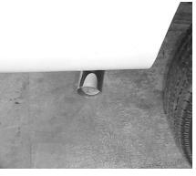
ADJUST TURNOUT PIPE SO IT EXITS THE SIDE OF THE VEHICLE AT A LEVEL POSITION. ONCE YOU HAVE EVERYTHING ADJUSTED AND HAVE CHECKED ALL CLEARANCES AROUND SPARE TIRE, SHOCKS, BRAKE LINES, ETC. TIGHTEN CLAMPS AT THE FRONT OF THE MUFFLER AND HEADPIPE. CHECK AGAIN FOR CLEARANCES THEN INSTALL YOUR STAINLESS STEEL TIP #H TO YOUR DESIRED LOOK. NOW TIGHTEN TAILPIPE AND TURNOUT PIPE. AFTER EVERYTHING IS TIGHT CHECK FOR CLEARANCES AGAIN.
