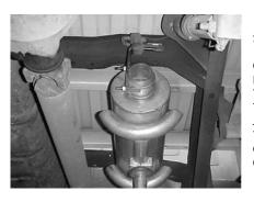
SLIDE MUFFLER#C, WITH INLET TOWARDS THE CONVERTER, OVER HEADPIPE #B NO LESS THAN 1 ½" AND NO MORE THAN 2". USE A JACKSTAND TO SUPPORT THE MUFFLER. CONNECT CLAMP #H TO MUFFLER OUTLET. DO NOT TIGHTEN. INSERT WELDED HANGER INTO RUBBER GROMMET.
