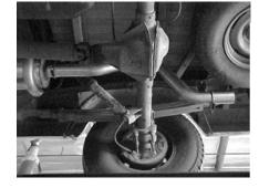
INSERT THE OVER AXLE TAILPIPE #D INTO REAR OF MUFFLER NO LESS THAN 1 ½" AND NO MORE THAN 2". CONNECT TO THE MUFFLER AND CLAMP USING #J. DO NOT TIGHTEN.
