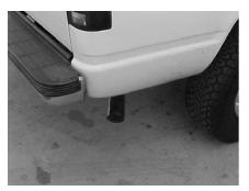
INSTALL STAINLESS STEEL TIP. CLAMP DOWN. TO CLEAN STAINLESS STEEL TIP USE STAINLESS STEEL OR ALUMINUM CLEANER. MAKE SURE YOU HAVE A **1" CLEARANCE ON** ALL PIPES FROM ALL RUBBER BRAKE LINES, FUEL LINES, SHOCK BOOTS, TIRES, ETC. WHEN YOU HAVE EVERYTHING IN PLACE, FIRMLY TIGHTEN ALL BOLTS AND CLAMP DOWN SECURELY.
