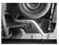
CONNECT TURNOUT EXIT PIPE #E TO THE REAR OF THE OVERAXLE PIPE. ROLL TURNOUT PIPE UNTIL YOU HAVE IT AT THE CORRECT ANGLE FOR YOUR TRUCK AND CONNECT CLAMP #1. DO NOT TIGHTEN.
