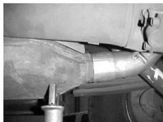
INSTALL OVERAXLE TAILPIPE # C ONTO OUTLET OF CONVERTER INSERT WELDED HANGER INTO RUBBER GROMMET.
