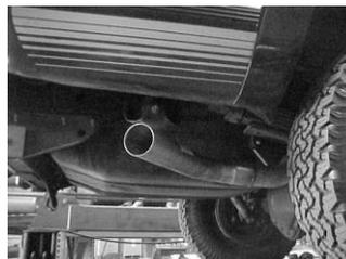
INSTALL EXIT PIPE #D ONTO TAILPIPE ROTATE UNTIL LEVEL. USE CLAMP # F TO SECURE PIPES TOGETHER. DO NOT TIGHTEN. WELD UP THE INLET & OUTLET ON THE CONVERTER.
