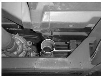
INSTALL HEADPIPE #A ONTO YOUR EXISTING STOCK FRONT PIPE AND SECURE WITH CLAMP #F. INSERT HANGER INTO RUBBER GROMMET. DO NOT TIGHTEN
