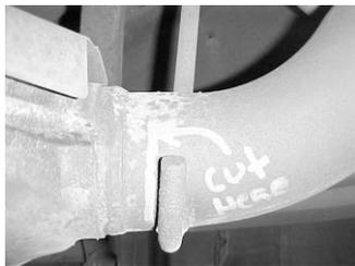
LAY OUT THE EXHAUST ON THE FLOOR SO IT LOOKS LIKE THE DRAWING AND COMPARE PARTS TO THE MANUAL. TO REMOVE THE STOCK EXHAUST CUT YOUR TAILPIPE OFF JUST BEHIND THE FACTORY HANGER. NEXT MEASURE 3/4" IN FRONT OF YOUR CONVERTER AND CUT, THEN UNCLAMP IT FROM THE CLAMP IN FRONT OF THE MUFFLER. THEN REMOVE THE STOCK MUFFLER AND EXTENTION PIPE. LEAVE ALL RUBBER GROMMETS IN PLACE. USE WD-40 TO AID IN REMOVAL OF HANGERS.
