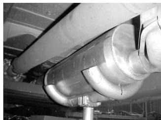
INSTALL MUFFLER #B ONTO HEADPIPE 1-1/2" TO 2" WITH THE LOUVERS FACING TOWARDS THE CONVERTER. USE A JACK STAND TO SUPPORT THE MUFFLER. USE CLAMP #F TO SECURE THE MUFFLER TO THE HEADPIPE. DO NOT TIGHTEN. MUFFLER INLET IS LOOKING INTO THE LOUVERS. OUTLET SHOULD BE AT THE 6 O'CLOCK POSITION.
