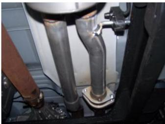
**3.** Install passenger side head pipe #A onto your existing stock front pipe and attach Flange with bolt kit #I. Do not tighten. Next, install driver side Headpipe #B onto stock pipe. Use clamp #H to secure together, do not tighten.
