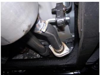
**6.** Install stainless steel tip. Clamp down. When you have everything in place, firmly tighten all bolts and clamps down securely. Use stainless steel cleaner and a Scotch Brite pad weekly to prevent tip from discoloration. Inspect all fasteners after 25-50 miles of operation and re-tighten as necessary
