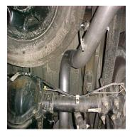
**7.** Install over axle tail pipe #C into muffler  $1\frac{1}{2}$ "-2". Use clamp #F to secure pipe to muffler. Do not tighten.
