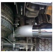
**8.** Slide exit pipe #D onto over axle tail pipe. Insert welded hanger into rubber grommet. Use clamp #F to secure pipes together. Do not tighten. Rotate pipe until level.
