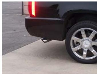
7. Install stainless steel tip #E. Clamp down. When you have everything in place, firmly tighten all bolts and clamps down securely. Use stainless steel cleaner and a Scotch Brite pad weekly to prevent tip from discoloration.
