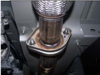
2. Remove the stock exhaust by removing it from the 2-bolt flange located in front of the muffler. Disengage the welded hangers using WD-40 from the OEM rubber grommets. Do not damage stock nuts and bolts or remove the rubber grommets as you will re-use them to mount your new system. Now, cut off tailpipe and remove exhaust.
