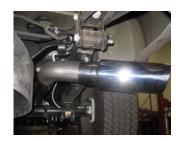
8. Install stainless steel tip. Clamp down. When you have everything in place, firmly tighten all bolts and clamps down securely. Inspect all fasteners after 25-50 miles of operation and re-tighten as necessary.
