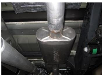
4. Install muffler #B onto headpipe #A 1.5-2" with louvers facing towards the converter. Use a jack stand to support the muffler
