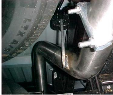
INSTALL THE OVERAXLE TAILPIPE #C INTO THE MUFFLER 1-1/2" TO 2". INSERT WELDED HANGER INTO RUBBER GROMMET. USE CLAMP #F TO SECURE TAILPIPE TO THE MUFFLER. DO NOT TIGHTEN.
