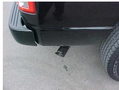
INSTALL STAINLESS STEEL TIP. WHEN YOU HAVE EVERYTHING IN PLACE, FIRMLY TIGHTEN ALL BOLTS AND CLAMP DOWN SECURELY. TO CLEAN STAINLESS STEEL TIP USE ANY STAINLESS STEEL CLEANER AND SCOTCH BRITE PAD.
