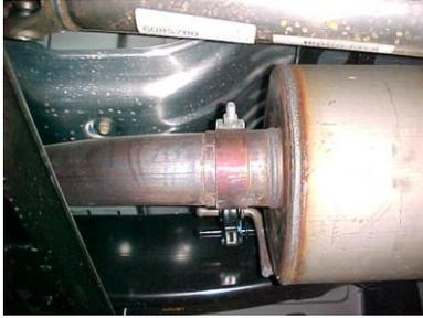
LAY OUT THE EXHAUST ON THE FLOOR SO IT LOOKS LIKE THE DRAWING AND COMPARE PARTS TO THE MANUAL. YOU MAY NEED TO HEAT IT UP FOR EASIER REMOVAL. LEAVE ALL RUBBER GROMMETS IN PLACE.
