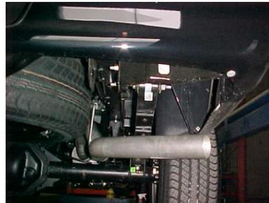
INSTALL EXIT PIPE #D ONTO OVERAXLE PIPE. ROLL TURNOUT PIPE UNTIL YOU HAVE IT AT THE CORRECT ANGLE FOR YOUR TRUCK AND CONNECT WITH CLAMP # F. BUT DO NOT TIGHTEN.
