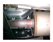
LAY OUT THE EXHAUST ON THE FLOOR SO IT LOOKS LIKE THE DRAWING AND COMPARE PARTS TO THE MANUAL. TO REMOVE THE STOCK EXHAUST UN-CLAMP IT JUST IN FRONT OF THE MUFFLER. DO NOT REMOVE THE STOCK HEADPIPE. YOU MAY NEED TO HEAT IT UP FOR EASIER REMOVAL. LEAVE ALL RUBBER GROMMETS IN
