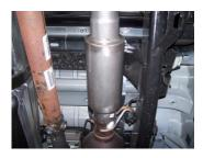
3. Slide muffler #A over stock headpipe 1.5-2". Use a jack stand to support the muffler. Use clamp #E to secure muffler to headpipe. Do not tighten.
