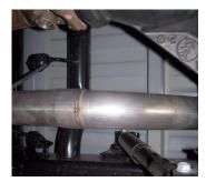
4. Slide extension pipe #B over muffler. Secure with clamp #E. Do not tighten. Insert welded hangers into rubber grommets.
