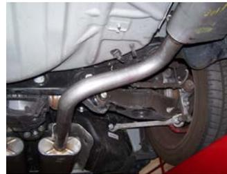
Now go back and make sure the first two mufflers in the middle are level. Then push up on factory cross member before tightening clamps. Then tighten X-pipe. Next, with both tailpipes in place tighten all bolts and clamps securely.
