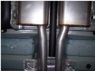
Install X-pipe assembly #A assembly on to your front factory pipes and secure with factory clamps. Re-install factory cross member. Use a jack stand to support mufflers. Do not tighten.
