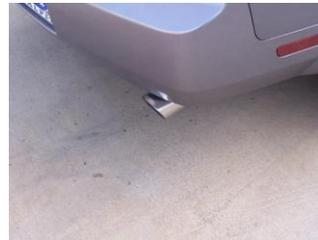
**4.** Install stainless steel tips. Clamp down. When you have everything in place, firmly tighten all bolts and clamps down securely. Use stainless steel cleaner and a Scotch Brite pad weekly to prevent tip from discoloration.
