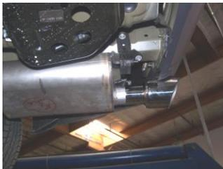
**2.** Install the factory grommets onto your Gibson muffler assembly as seen in the picture.
