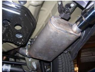
**3.** Install muffler assembly onto factory pipe, use clamp #B to secure. **DO NOT TIGHTEN.** Next tighten grommets to frame and adjust muffler assembly.
