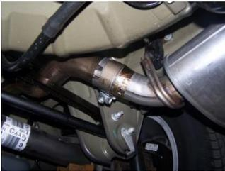
**1.** Remove your stock assembly from the clamp located in front of your stock muffler, unbolt the factory hangers from the frame.
