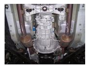
4. Now disconnect all 3 sensors on the stock h-pipe with a 22mm wrench. Once you have done that, then unbolt the flanges at the stock manifolds and slide h-pipe out of rubber grommets. Save all stock hardware and clamps. You will re-use them later.
