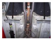
7. Install the passenger side tailpipe #B into muffler assembly using clamp #E to secure. Do not tighten. Now do the same procedure for the driver side tailpipe. Use clamp #E to secure the tailpipe to the muffler assembly. Now use the stock clamps to secure the tailpipes to the X Pipe.
