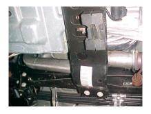
INSTALL PIPE #I ONTO PIPE #J. USE CLAMP #E TO SECURE PIPES TOGETHER. DO NOT TIGHTEN.
