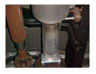
Install head pipe # A on to your stock catalytic converter and line up the notch. Then secure with clamp #E. Insert hanger into rubber grommets. Do not tighten.
