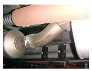
LAY OUT YOU GIBSON EXHAUST ON THE FLOOR SO IT LOOKS LIKE THE DRAWING AND COMPARE PART #'S TO THE MANUAL. TO INSTALL YOUR GIBSON DOWN PIPE YOU NEED TO REMOVE YOUR STOCK EXHAUST. REMOVE THE STOCK EXHAUST FROM THE **CLAMP LOCATED JUST** BEHIND THE CATALYTIC CONVERTER. CUT OFF YOUR STOCK TAILPIPE FOR EASIER REMOVAL. LEAVE ALL RUBBER GROMMETS IN PLACE. USE WD-40 TO AID IN REMOVAL OF EXHAUST AND HANGER
