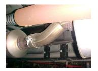
Lay out the exhaust on the floor so it looks like the drawing and compare parts with manual. To remove the stock exhaust remove it from the clamp located just behind the catalytic converter. Cut off your stock tailpipe just behind the muffler for easier removal. Leave all rubber grommets in place. Use WD-40 to aid in removal of exhaust and hangers.
