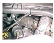
4. Remove the remaining stock downpipe by unclamping it from the turbo housing. Use an 11mm socket or wrench to remove your stock pipe through the bottom. Do not discard the stock you will need to reuse it. Now, install downpipe #A onto turbo reusing your stock clamp. Do not tighten.
