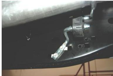
REMOVE THE HANGER FROM THE FRAME AND RELOCATE TO THE HOLES JUST TO THE LEFT OF THE OTHER HOLES. YOU WILL NEED TO PRY THE INSERTS OUT AND RE-INSTALL. SEE PHOTO.
