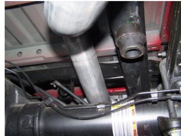
INSTALL OVERAXLE TAILPIPE #C INTO MUFFLER 1 1/2" TO 2". INSERT HANGERS INTO RUBBER GROMMETS. USE CLAMP #E TO SECURE PIPE TO MUFFLER. DO NOT TIGHTEN.
