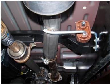
INSTALL HEADPIPE # A INTO STOCK PIPE. THE END OF THE PIPE SHOULD BE AT THE 12 O'CLOCK POSITION., INSERT WELDED HANGERS INTO RUBBER GROMMET. ATTACH WITH FACTORY CLAMP. DO NOT TIGHTEN. REMOVE THE HANGER FROM THE FRAME & RELOCATE TO THE HOLES JUST TO THE LEFT OF THE OTHER HOLES YOU WILL NEED TO PRY THE INSERTS OUT & RE-INSTALL SEE PHOTO
