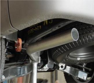
INSTALL EXIT PIPE #E AND INSERT WELDED HANGER INTO RUBBER GROMMET.
