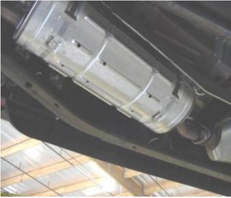
TO REMOVE STOCK EXHAUST UNBOLT IT FROM THE SLIP-FIT JOINT LOCATED IN THE REAR ABOVE THE AXLE AND SLIDE THE TAILPIPE OUT. NEXT UNBOLT THE 2-BOLT FLANGE LOCATED JUST BEHIND THE CATALYTIC CONVERTER. **DO NOT THROW AWAY STOCK NUTS AND BOLTS YOU WILL NEED TO RE-USE THEM.** NOW CUT OFF YOUR STOCK TAILPIPE JUST BEHIND THE MUFFLER AND REMOVE. LEAVE ALL RUBBER GEOMETTS ON THE HANGER. USE WD-40 TO AID IN THE REMOVAL OF EXHAUST AND HANGERS.
