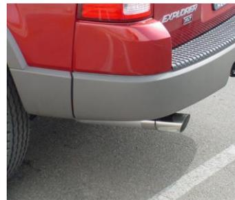
INSTALL THE STAINLESS STEEL TIP. TO CLEAN TIP USE ANY ALUMINUM OR STAINLESS CLEANER AND A SCOTCH BRITE PAD. GO BACK AND TIGHTEN ALL NUTS, BOLTS AND CLAMPS STARTING IN THE FRONT AND WORKING BACK.
