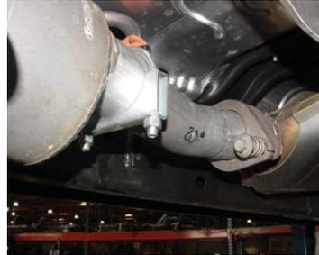
SLIDE FLANGE #A OVER GIBSON HEADPIPE #B. SLIDE HEADPIPE INTO MUFFLER 1-1/2" TO 2" USE CLAMP #H TO SECURE HEADPIPE TO MUFFLER. DO NOT TIGHTEN. NEXT USE YOUR STOCK NUTS AND BOLTS TO SECURE HEADPIPE TO STOCK FLANGE.
