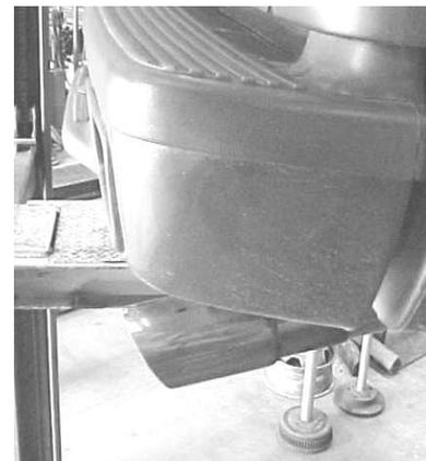
INSTALL THE STAINLESS TIP. USE ANY ALUMINUM OR STAINLESS STEEL CLEANER TO POLISH YOUR STAINLESS STEEL TIP. NOW GO BACK AND TIGHTEN THE FLANGE AT THE CATALYTIC CONVERTER, HANGER AND CLAMPS.
