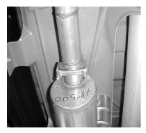
NEXT INSTALL THE HEADPIPE #A ON TO THE FACTORY FLANGE USING FLANGE #E AND RE-USING THE STOCK BOLTS. DO NOT TIGHTEN. INSTALLTHE MUFFLER #B WITH INLET FACING FORWARD. THE INLET OF THE MUFFLER WILL HAVE THE LOUVERS FACING FORWARD CATCHING THE EXHAUST GOING IN. MUFFLER INLET IS LOOKING INTO THE LOUVERS. ATTACH MUFFLER TO HEADPIPE WITH CLAMP #G. THE MUFFLER OUTLET WILL BE POSITIONED AT ABOUT 6 O'CLOCK.
