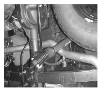
INSTALL THE OVERAXLE PIPE #C INTO THE OUTLET OF THE MUFFLER. SLIP THE OVERAXLE PIPE HANGER INTO THE REAR RUBBER GROMMET. INSERT WELDED HANGER INTO RUBBER GROMMET.
