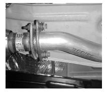
LAY OUT THE GIBSON EXHAUST SO IT LOOKS LIKE THE PICTURE AND COMPARE THE PART NUMBERS TO THE MANUAL TO MAKE SURE YOU HAVE THE CORRECT PART NUMBERS. THEN REMOVE THE FACTORY EXHAUST. FOR AN EASIER REMOVAL OF THE EXHAUST CUT JUST BEHIND THE MUFFLER ON THE TAIL PIPE. THEN UN-BOLT THE FACTORY FLANGE IN FRONT OF THE STOCK MUFFLER. YOU WILL RE-USE THE STOCK FLANGE BOLTS. NOTE: LEAVE ALL RUBBER GROMMETS IN PLACE
