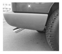
NOW INSTALL YOUR STAINLESS STEEL TIP TO YOUR DESIRED LOOK. USE ANY ALUMINUM OR STAINLESS STEEL CLEANER TO POLISH YOUR STAINLESS STEEL TIP. THEN TIGHTEN THE HEADPIPE. CHECK CLEARANCE AGAIN. NOW TIGHTEN ALL HANGERS AND CLAMPS.
