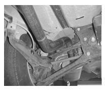
2.) INSTALL REAR EXTENSION PIPE # C. USE CLAMP # G TO ATTACH IT TO THE RESONATOR. DO NOT TIGHTEN.
