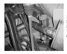
3.) INSERT THE WELDED HANGER ON THE REAR EXTENSION PIPE #C INTO THE REAR RUBBER GROMMET.
