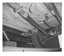
1.) INSTALLTH E FRONT EXTENSION PIPE #B. INSTALL THE FRONT RESONATOR #A. NOTE: THE LOUVERS ON THE INSIDE OF THE RESONATOR WILL BE FACING FORWARD TOWARDS THE ENGINE. USE A JACK STAND TO SUPPORT THE RESONATOR.
