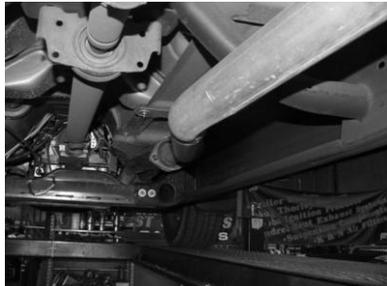
TO REMOVE STOCK EXHAUST UNBOLT IT FROM THE FLANGE LOCATED JUST BEHIND THE FACTORY Y-PIPE. **YOU WILL RE-USE YOUR FACTORY BOLTS FROM FLANGE.** NOW, CUT OFF YOUR STOCK TAILPIPE JUST BEHIND THE MUFFLER AND REMOVE. LEAVE ALL RUBBER GROMMETS ON THE HANGER. USE WD-40 TO AID IN REMOVAL OF THE EXHAUST AND HANGERS.
