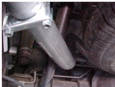
INSTALL DRIVER SIDE TAILPIPE #D, INTO MUFFLER AT LEAST 1 1/2" TO 2". THIS PIPE WILL ROUTE OVER THE AXLE AND BETWEEN THE SHOCK AND TIRE. ATTACH CLAMP #I TO SECURE TAILPIPE TO MUFFLER. DO NOT TIGHTEN. LOOKING FROM THE REAR OF THE VEHICLE – THIS TAILPIPE IS AT APPX. 11 O'CLOCK.
