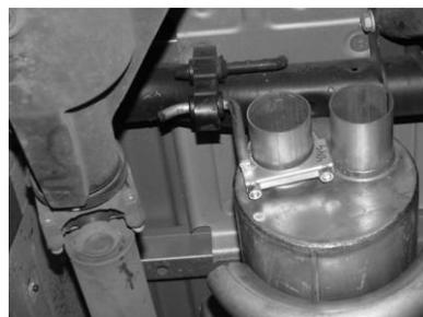
INSTALL MUFFLER #B ONTO HEADPIPE, AT LEAST 1 1/2" TO 2". USE CLAMP #F TO SECURE MUFFLER TO HEADPIPE. DO NOT TIGHTEN. USE A JACK STAND TO SUPPORT THE MUFFLER. OUTLETS SHOULD BE AT THE TOP. INSTALL REAR MUFFLER HANGER #I ONTO DRIVERSIDE MUFFLER OUTLET AND INSERT WELDED HANGER INTO GROMMET. DO NOT TIGHTEN.
